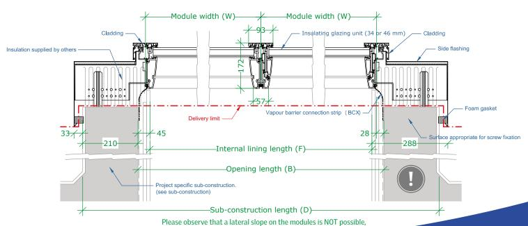
therefore top and bottom sub-construction must be horizontal.
